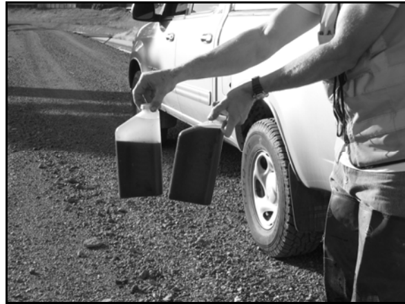
Figure 5. Water samples from Putah South Canal collected during 2007 cleanout. The sample on the right was just collected; the sample on the left had settled for about 30 minutes. Both samples contain high concentrations of organic materials (decomposed vegetative materials) with a little sediment.
