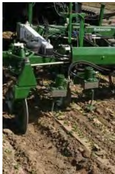
Figure 1. Tillet cultivator. Note blade on the right is elevated to show the pie shaped design that allows the blade to spin around the crop plant as it travels down the seedline.
