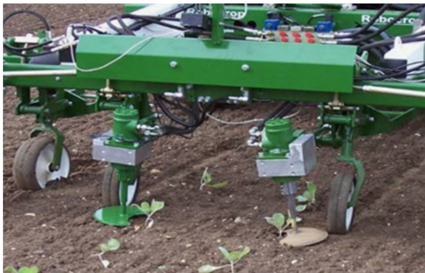
Fig. 1. The Tillet Weeder is a commercially available mechanical weed control machine that uses computer technology and a spinning blade to remove weeds. Note the disc-shaped cultivation blade with a notched cut-out to allow the blade to spin around transplanted cabbage.
