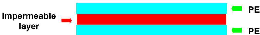
Figure 3. Impermeable film consists of at least three layers. In the three layer film shown above, the top and bottom layers consist of normal polyethylene tarp, and the middle layer consists of an impermeable layer.
