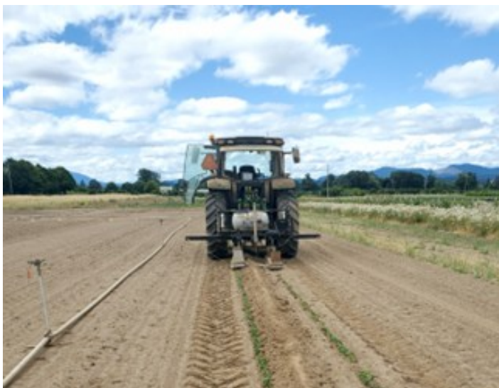
Figure 2. Two-row flamer used in the study to apply over the crop rows in trial 1. The snap beans emerged to early and were larger than the weeds at time of application leading to significant injury on the beans.
