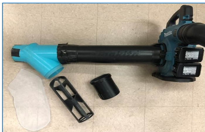
Photo 1. Modified Makita blower/vacuum complete with 3D printed parts and custom mesh bags for collecting arthropod samples.
